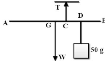
In the figure, AB is a meter scale of weight  $W$  which acts at the centre of gravity  $G$  (50 cm mark). The 50 g weight is suspended at  $D$  (75 cm mark) and the scale balances at  $C$  (60 cm mark). Let  $T$  be the tension in the string (in gram weight). Consider the equilibrium of the scale at the point  $C$  and applying the conditions for equilibrium,
