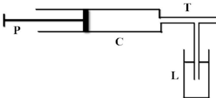
The figure shows the essential parts of an atomiser.  $C$  is a cylindrical barrel which terminates in a small tube  $T$ .  $T$  is connected to a vessel  $L$  containing the liquid to be sprayed. When air in the barrel is pushed by the piston  $P$ , the speed of the air increases considerable in tube  $T$ . According to Bernoulli's principle, this causes a reduction in pressure. As a result, the liquid in the vessel rushes up and mix with high speed air to form a fine spray.
